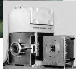
left: Longitudinal flux testing with ROTOMAT right: Transverse flux testing with TRANSOMAT integrated in multi-test block – in this case at Vallourec Mannesmann in Belo Horizonte, Brazil, for seamless tubes up to 168.3 mm diameter and 12.7 mm wall thickness.
